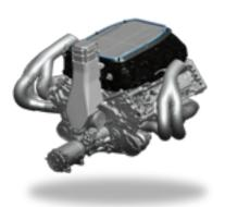
For a third consecutive year, Scuderia Toro Rosso's motive power comes from a short drive up the Autostrada in Maranello. The Ferrari V10 retains the same 056 code number, as a result of the engine freeze, but with new rules concerning how many engines can be used, a reduction in the maximum rev limit and the need to cope with the arrival of KERS, the engine engineers have had plenty to think about while preparing for the 2009 season.
